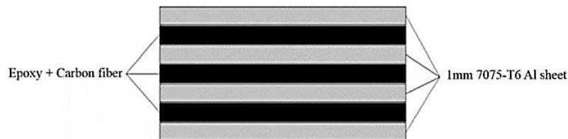
Fig 1. The sequence of the composite material produced is given schematically.
