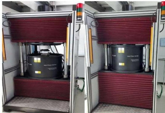
Fig 5. Hot pressing device used in composite production.
