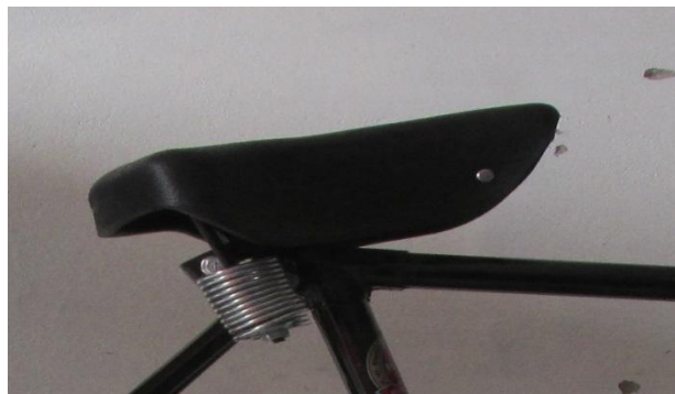
Fig 1. Seat arrangement and suspension spring
