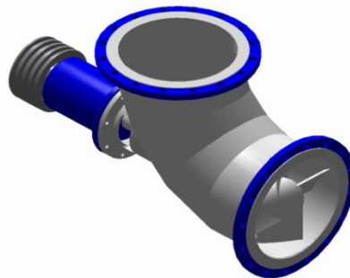
Fig 7. Axial flow pumps
